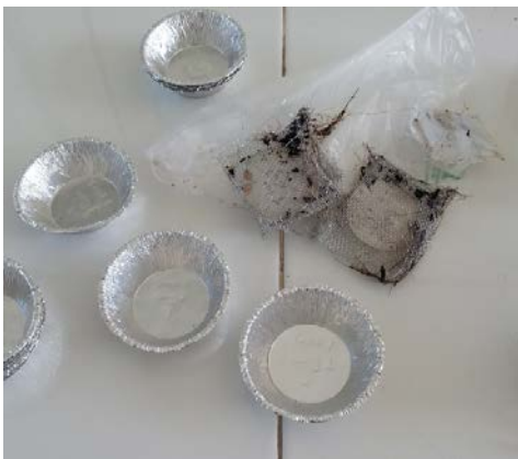
Figure 6. Aluminium tins used when drying the glass filter in the oven and the net cages, still with filters inside.
