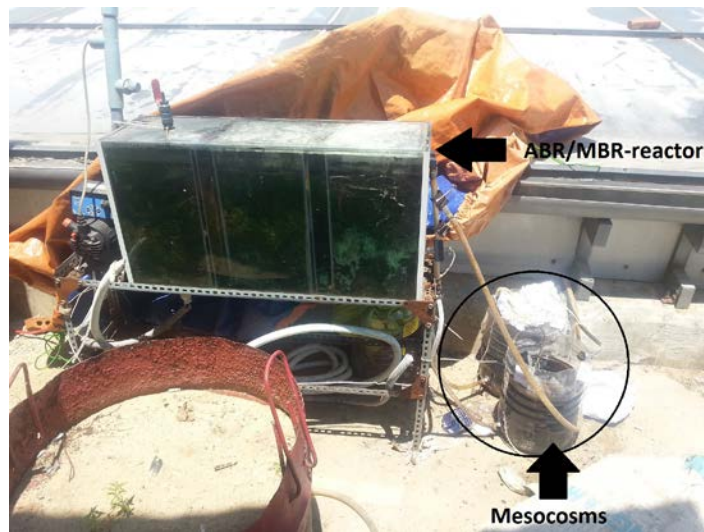
Figure 5. The actual prototype ABR/MBR-system together with the mesocosms. The picture shows how the hose connects the ABR/MBR-system to the bottom of the tanks containing nutrient reduction materials.
