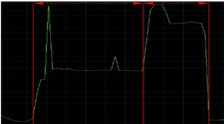
**Figure 4. Wave of the current consumption of sending one packet with Z-Wave. First part from the first red line to the second redline is the startup of the Z-Wave, and the second part starting from the second red line to the third red line is the consumption when sending data.**
