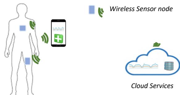
Figure 1. Placement of inertial measurement sensors
