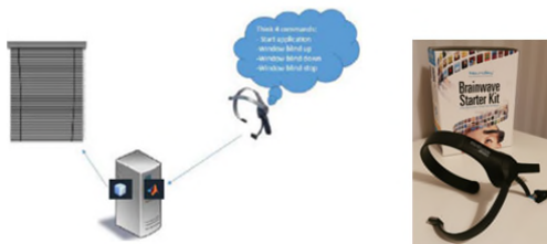
Figure 5. The NeuroSky BrainWave Headset.
